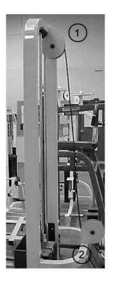
Figure 7. Upper and lower pulleys.
